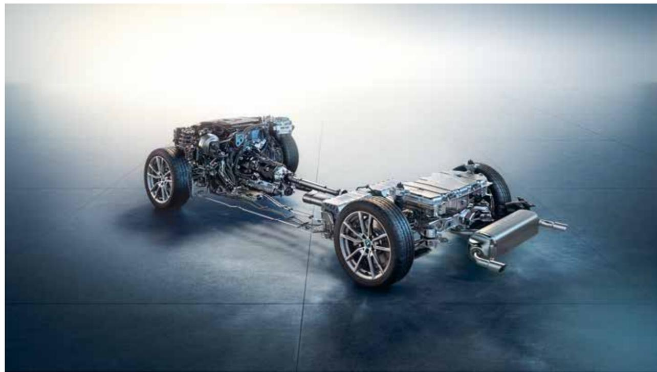
The intelligent **BMW xDrive all-wheel drive system** continuously and variably distributes the drive force to the front and rear wheels – for increased traction, driving dynamics, directional stability and driving safety in every traffic situation.
