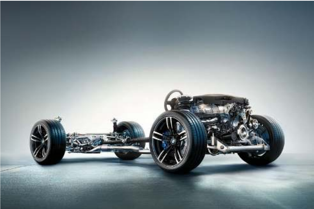
Thanks to the use of different materials, M compound brakes achieve outstanding deceleration values and are extremely stable and highly durable. They also weigh less, which has a positive impact on agility, dynamics and acceleration. The Blue metallic brake callipers with the M logo are the hallmark of these high-performance compound brakes.
