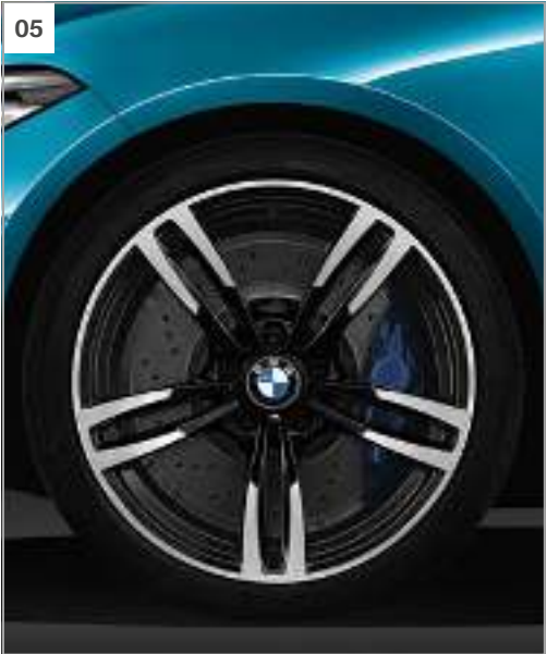
[ 05 ] 19" M light alloy wheels Double-spoke style 437 M with non-run-flat mixed tyres, gloss-lathed, forged, black, front 9 J x 19 with 245/35 R 19 tyres, rear 10 J x 19, with 265/35 R 19 tyres.
