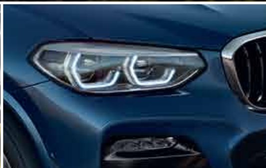
BMW Icon Adaptive LED Headlights with BMW Selective Beam incl. LED Fog lights.
