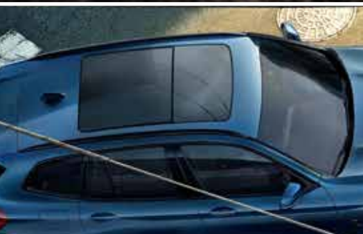
Panorama glass roof, with electric operation of glass roof and sun protection roller blind.
