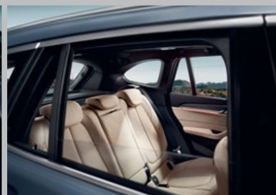
Adjustable backrest in 6 tilt positions incl. fore-and-aft adjustment
